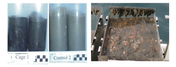
**Figure 4** Mud samples from beneath salmon cages in the Marlborough Sounds. Left: black anoxic sediments from beneath cages compared with brown sediments from a control site beyond the influence of the farm. Right: sediment grab sample with black sediment and faecal material (orange) evident.
